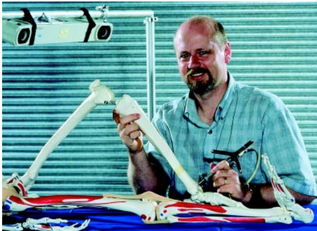
Dr. Hodgson demonstrates the use of an optoelectronic localizing probe to find the anatomic centre of the ankle during a mock-up of a computer-assisted knee replacement procedure. A current project in his lab aims to replace this anatomic digitization with a kinematic analysis of the ankle joint motion
